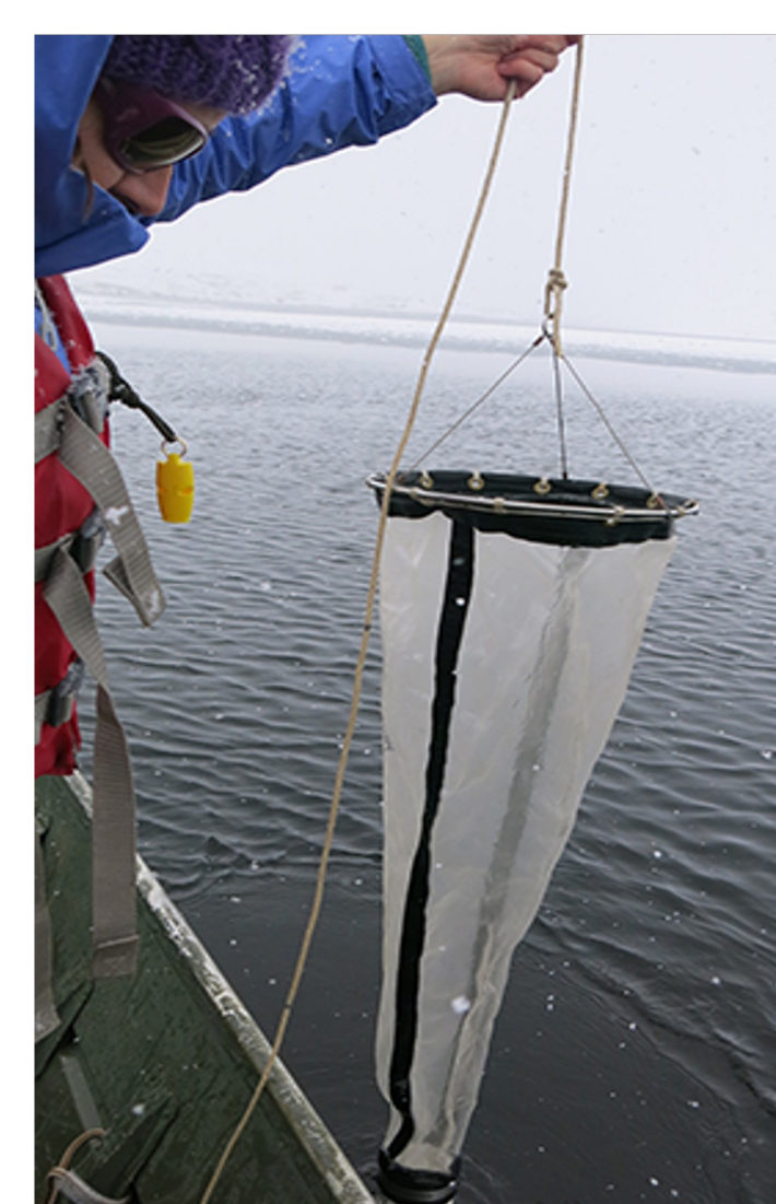
Figure 4. Zooplankton net used to collect samples of zooplankton.
